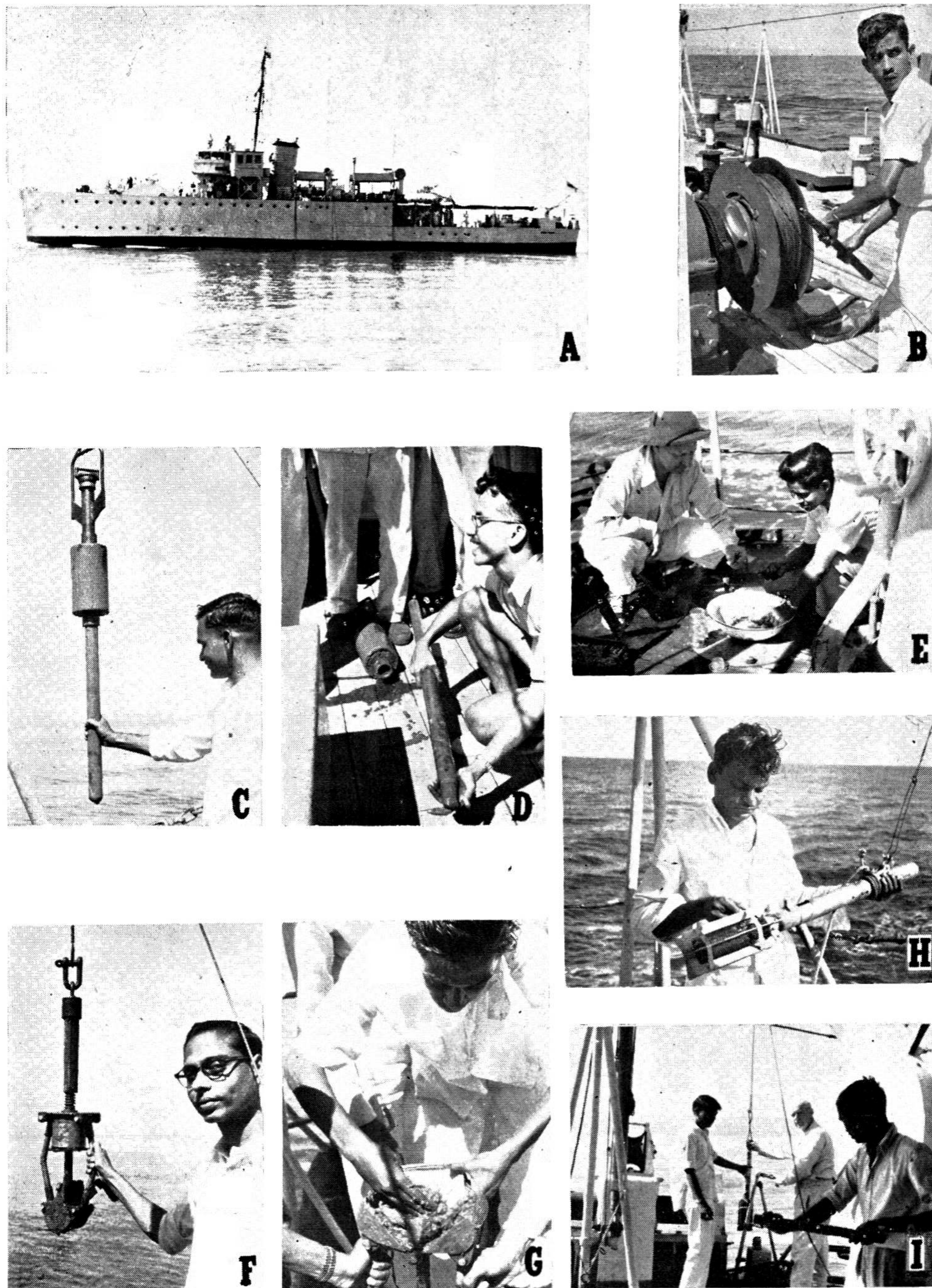
FIG. 2. Oceanographic equipment and measurements. (A) I.N.S. Rohilkhand used for oceanographic work. (B) Level-winding wire rope on electric winch drum. (C) Retrieving Phleger corer. (D) Extracting sea floor sediment core from corer. (E) Examining marine samples. (F) Retrieving sea floor sediment snapper. (G) Extracting sediment from snapper. (H) Placing glass slide in bathythermograph for temperature. (I) Lowering bathythermograph off stern of ship.
